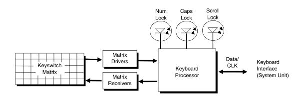
Figure C-1. Keystroke Processing Elements, Block Diagram
